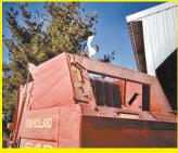
A length of angle iron bolts onto the ejector's frame. A 3/8-in. dia. metal rod attaches to the angle iron and extends through the baler housing to the front part of the baler where an old handkerchief is tied onto it.
