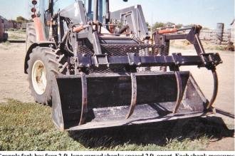
Grapple fork has four 2-ft. long curved shanks spaced 2 ft. apart. Each shank measures 1 in. thick by 2 in. wide.
