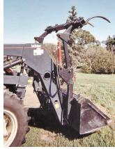
David McKenzie used old cultivator shanks to build heavy duty, loadermounted grapple forks. They mount on a Zetor tractor equipped with a Buhler front-end loader.
