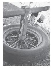
A 12-in. length of the axle sticks up out of the 36-in. dia. wheel's hub (left). Home-made handlebars at the end of the pipe are welded to an adjustable sleeve (right).
