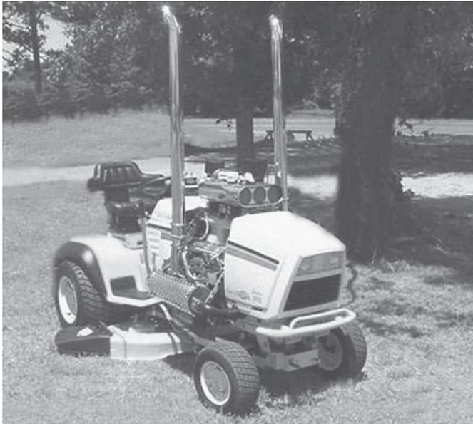
"I call it the Cub Ca-Debt because I probably have \$15,000 to \$20,000 invested in materials alone," says Avery Allred. It's got a Chevy truck engine block, but all of the internal components were hand molded, cast and fabricated including the camshaft and engine timing gears.
