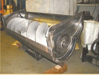
Blower's 15-in. dia. auger rotates at 1,050 rpm's, powered by Deere's front drive system. Clearances between the auger and housing are less than 1/10th in.
