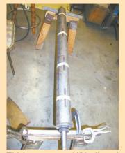
Flighting mounts on a 1.25 in. dia. steel shaft fitted with a 4-in. dia. center pipe. Gerken balanced it as he went along with small pieces of steel stock.
