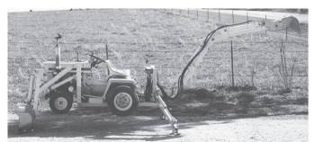
Loader is made from 1 by 2-in. heavy wall rectangular tubing. Its bucket measures 38 in. wide and is made from 3/16-in. thick steel plate. Backhoe bucket measures 8 1/2 in. wide and is tilted up or down by a 3 1/2-in. dia. cylinder.
