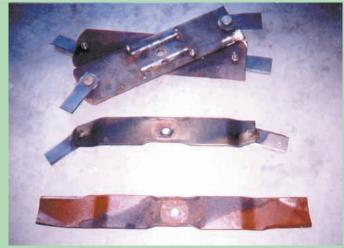
Top blade is an experimental one while bottom blade is an original untouched blade. Gallaher says the simplest arrangement - the middle blade - works best.
