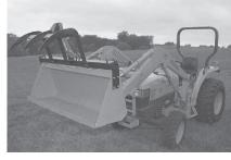
Grapple fork fits compact tractors with a 5 or 6-ft, wide bucket. It comes with a telescoping mounting frame that attaches to each side of the bucket. The frame is designed to accept either single or double grapples. A single grapple sells for \$500; a double for \$850.
