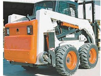
Each wheel is attached to a hydraulic cylinder that operates off skid loader’s remote outlets. By flipping a switch inside the cab, you can lower the wheels to raise the rear skid steer wheels up to 1 1/2 in. off the floor. Wheels lift up out of the way when not needed.
