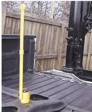
Upright poly pole fits over hitch ball. As you back up you line up the gooseneck until it just touches the hitch guide. Then you remove the hitch guide and lower the gooseneck onto the ball.
