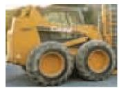
Sylvan Yoder mounted big 24-in. high wheels on this Case 95XT skid loader to speed it up. "With the transmission in high range the loader can go 18 mph, which compares to about 10 mph with conventional wheels," he says.
