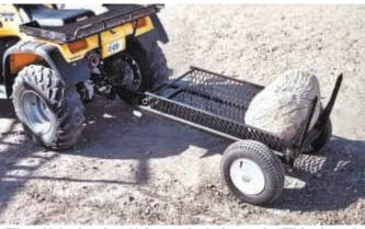
ATV towable hand cart has a hitch on top that hooks up to the ATV drawbar, and a pair of adjustable prongs to load rocks.
