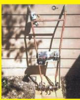
Here's a cultivator I made for tilling in between rows of vegetables. I made some tines out of stainless steel and mounted them between the handles off an old mower. The tines are powered by a 1/2 in. cordless drill that chain-drives the tines. Instead of wheels, I put two skids on it. *(Ken Voigt, Wausau, Wis.)*
