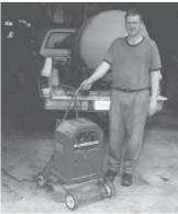
Dennis and Roger Koelling, Bartelso, Ill.: "By mounting our Lincoln AC-DC electric welder on the deck of an old 22-in. push mower, we can easily move the welder anywhere inside our shop.
