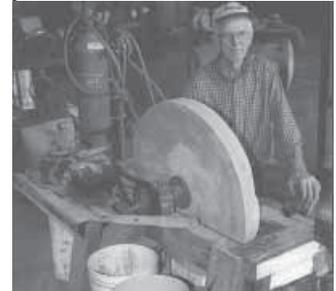
**Noel Hicks, Palmyra, Ill.:** He took an old foot-powered grindstone, built a stand for it and motorized the grindstone. It works a lot better than modern high-speed grinders because it grinds slowly and doesn't burn the edges as fast, says Hicks.
