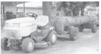
Hauler consists of a two-wheeled trailer that hooks up behind the tractor and a dolly
