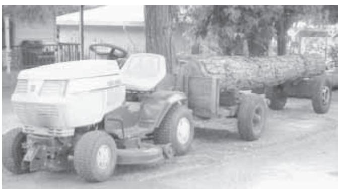
Hauler consists of a two-wheeled trailer that hooks up behind the tractor and a dolly that holds the back end of the log.
