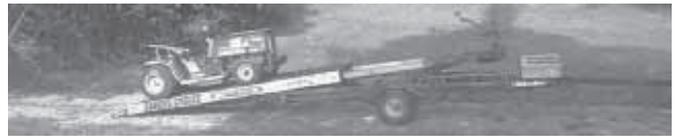
Trailer has an 8-ft. long, 5-ft. wide expanded metal deck that moves forward or backward up to 7 ft.
