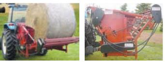
BeddingPro bale shredder attaches to a 3-pt. hitch or quick-taches to a front-end loader. It shreds and fluffs straw so well livestock producers can extend bedding intervals, says manufacturer Paul Fox.
