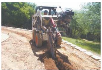
Jeff Craig built a trencher for his skid steer loader, starting with an old trencher chain he found in the dumpster at a Bobcat dealer.
