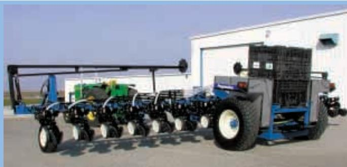
**Instead of a seed hopper, Rich Follmer's new planter has an air delivery system that takes seed directly from bulk boxes to planting units.**
