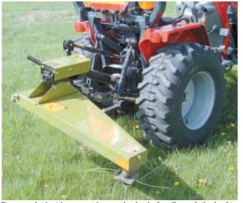
$\label{thm:condition} \textbf{Pto-powered string trimmer can trim around and under fence lines and other hard-to-cut areas.}$
