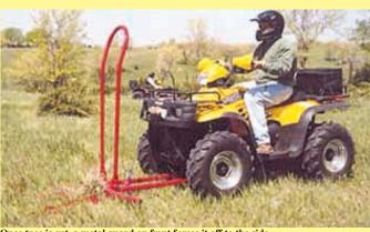
Once tree is cut, a metal guard on front forces it off to the side.
