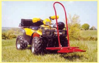
ATV-mounted "Tree Chopper" lets you cut down small trees on-the-go. It slices through trunks up to 4 in. in diameter, yet requires no outside power source.
