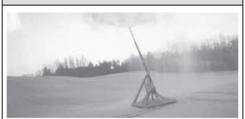
A high-pressure pump feeds well or pond water to this 22-ft. tower-type snowgun.
