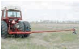
Clipper is available for both front and rear 3-pt. mounting. The rear model can be easily towed behind a pickup with a receiver hitch.
