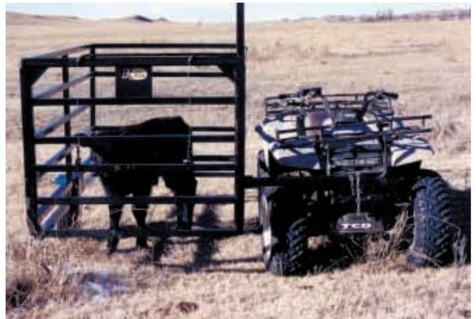
Calf catcher bolts onto one side of ATV. To catch a calf, driver approaches it with door open. Once calf is inside corral, he lets go of a rope to shut the door.
