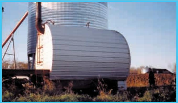
Bale furnace mounts on trailer so it can be easily moved to anywhere it's needed.
