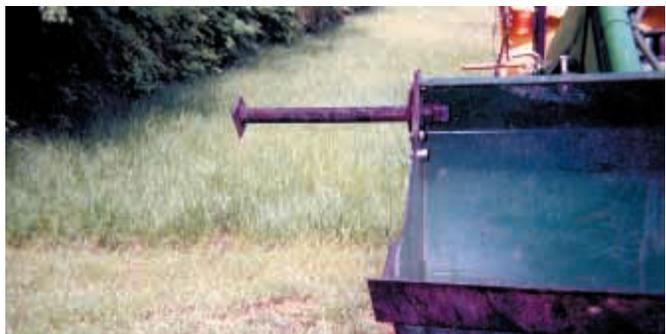
A roll of wire simply slips onto pipe mounted on side of loader bucket.
