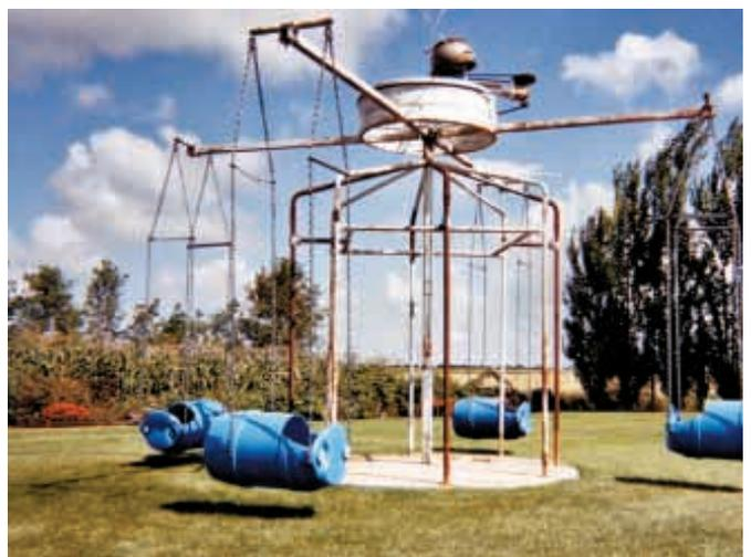
Four 30-gal. plastic barrels, attached by lengths of chain to arms, go "flying" as the arms rotate.
