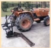
T.E. Salsman converted a 43-in. sicklebar and gearbox from an older walking mower to mount on his Kubota tractor. Gearbox is chain-driven by a hydraulic motor.
