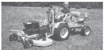
By turning a Cub Cadet garden tractor around and mounting a 48-in. deck on front, Jon Whitledge was able to convert it into this low-cost zero turn mower.
