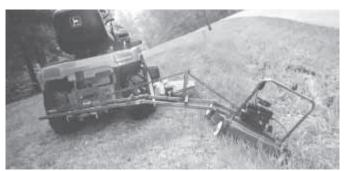
Homemade flexible hitch allows Chris Rahman to pull a 22-in. push mower 2 ft. to the side of his Deere garden tractor.
