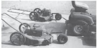
Darrell Demaray pulls two 22-in. push mowers behind his 48-in. Deere all-wheel steer riding mower. Each mower hooks to a single 8-in. high caster wheel on front.
