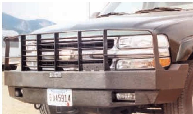
**Grill is coated with spray-on pickup bed liner to keep rocks and debris from chipping the surface.**
