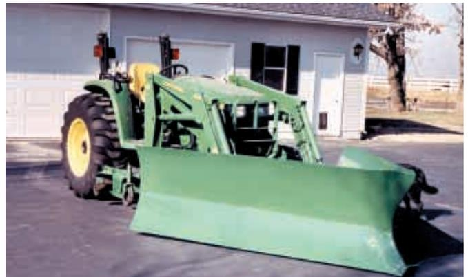
V-blade is 3/16-in. steel that is 30 in. high and 8 ft. long. A 5-in. curve keeps snow from riding up over blade.
