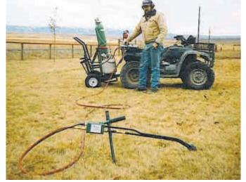
Remote control allows Shaffer to detonate gas from up to 25 ft. away.
