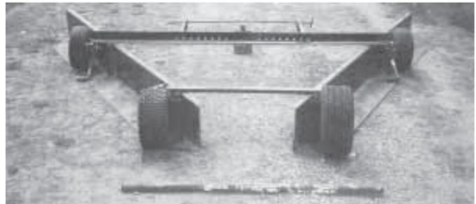
Harley Windrower can be mounted under any tractor or used as a pull-type to clear 8 to 10-ft. swaths of ground at a time.
