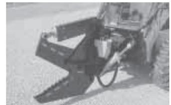
Teeth added to stationary side of shear dig into tree trunk as blade begins to close, preventing slippage.
