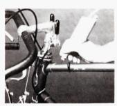
Rockwell engraver has a replaceable carbide point, adjustable depth of cut and a pencil-type grip for sure control.
