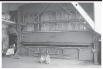
Brake press measures 15 ft. high and has a 20-ft. wide bed. It weighs about 18,000 lbs.
