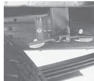
When you're not hauling a heavy load, the Loadhelper can be raised up and the pickup will perform normally.
