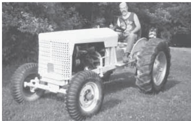
It has the hood and grill from a Cletrac bulldozer, the engine from a 1/2-ton Chevy pickup, and many other parts, says Eric Lindroth about his home-built tractor.
