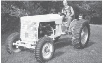
It has the hood and grill from a Cletrac bulldozer, the engine from a 1/2-ton Chevy pickup, and many other parts, says Eric Lindroth about his home-built tractor.
