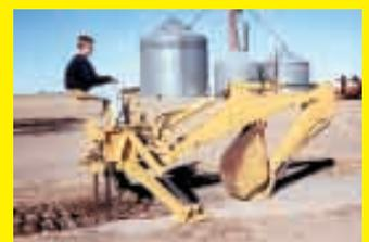
designed to be an integral unit. We made adapter couplers that let us hook the backhoe onto our tractor's 3-pt. We also reworked the hydraulic system so it would
