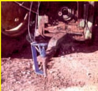
a 13 1/2-in. long, U-shaped handle on one side. The tractor driver simply pulls on a rope to release the handle, and then pulls the pin out of the drawbar. A rotating collar at the top part of the handle allows the pin to rotate so the handle won't twist off while hauling heavy loads. I've made a few sets of both the steps and drawbar pins for neighboring farmers. (Brian Lexvold, 30380 Hwy. 19 Blvd., Red Wing, Minn. 55066 ph 651 388-3883)
