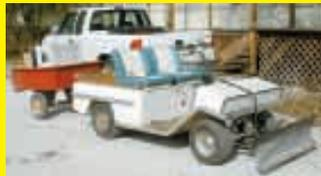
I got tired of taking the mower deck off my Murray lawn tractor every fall and putting on the snow plow for the winter. So I converted an old electric golf cart to do my snow plowing and to grade my driveway. I made an angle iron bracket and bolted it onto the frame under the hood. The snow blade bolts onto this bracket with two bolts, so it takes only a couple of minutes to mount the blade. But it's so handy that I never take it off.
