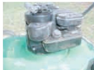
Second starter mounts in slot cut into shroud on carburetor side of motor.
