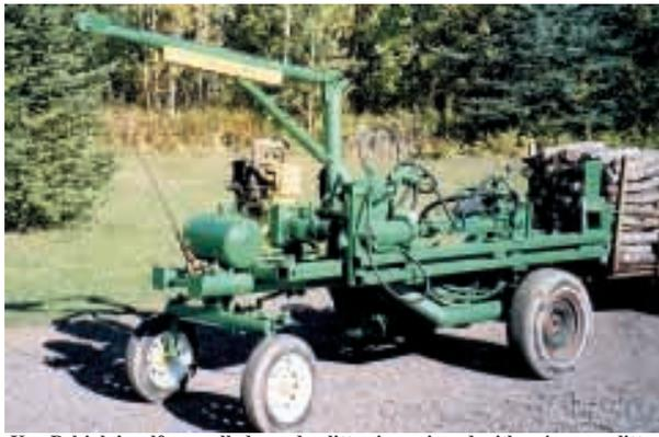
Ken Pohjola's self-propelled wood splitter is equipped with a 4-way splitter on back and a winch and lift boom on front.
