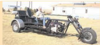
Two up-front chrome springs and two air bags support the 5.9-liter Cummins diesel engine. Both the engine and transmission came out of a 1991 Dodge pickup.
