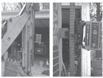
James Boyd used parts from a garage door opener to come up with this low-cost grade sensor for his backhoe. He uses it when installing field tile.
