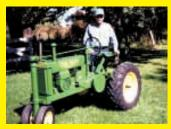
steering post was cut down from a Deere H. The cap on the air intake was a soup ladle. The top of the radiator was routed out of solid mahogany by my son. It's not a kit. I made most of the parts myself using a chop saw.
