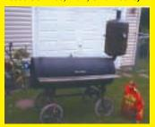
I made this BBQ "smoker" from half of an old 80-gal. electric water heater. Electric heaters are the best because they don't have flue pipes through the center. Water heaters have a glass lining so they won't rust through. (Tom Belusko, 2451 Hemlock Ave., Granite City, III. 62040 ph 618 797-2016).
