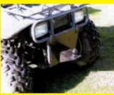
small spaces. So I got my stick welder and a bunch of scrap metal and made a bracket that slips on front of my ATV. The bracket is equipped with a ball hitch and
