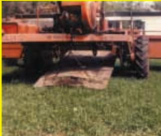
pair of homemade steel brackets about 4 ft. apart on back of the swather frame. The roller hangs from the brackets via two chains, one at each end of the roller. I adjust the chains to control the height of the roller. I used 1 1/2-in. sq. steel to make the uprights for the bracket, and 1-in. sq. steel for the rest of it.
