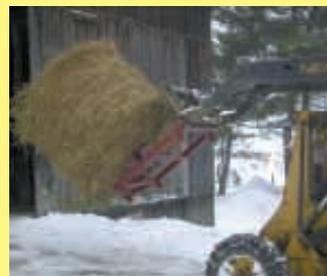
Spinner attaches to loader arms and is used to pick up bale.
