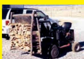
I used 3-in. dia. wood poles to make a firewood rack that I move around with a small loader tractor. The firewood rack has a pair of A-shaped uprights at each end that are lashed together with wire. A horizontal pole on top is lag screwed to the uprights. The floor consists of more horizontal poles. To haul wood I simply position the loader bucket underneath the horizontal pole on top, then raise the bucket and drive off. **(Bob Barnes,**
