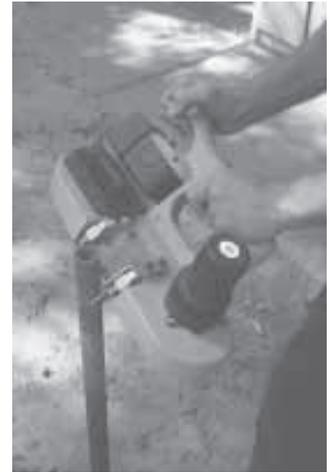
**Bandsaw is 15 in. long, weighs 8 lbs. and is light enough to hold in one hand.**
