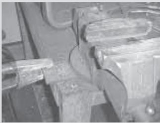
"I do most of my welding at my bench vise. I added a lug to one of the vise's hold-down bolts to securely attach a ground."
