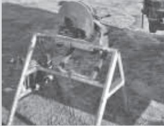
saw mounts on a hinged metal rack that's welded to the top part of the saw horse. Both the rack and chop saw swing down out of the way when not in use. The sawhorse has an electric outlet on it with an extension cord wrapped around it to provide electricity. To use the chop saw I just unroll the cord and plug it into the chop saw.
