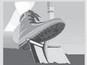
magazine. You can give your shovel-shoving foot a more comfortable pushing surface by cutting a slit in a scrap of 1-in. pvc pipe and slipping it over your shovel's flange. If it won't stay put, just add a bead of hot-melt glue.
