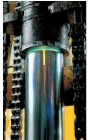
Tracerline leak detection can be used on virtually any fluid, including water and other clear liquids.
