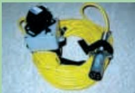
Insulated electric cord connects both sensor and light to lower end of auger.
