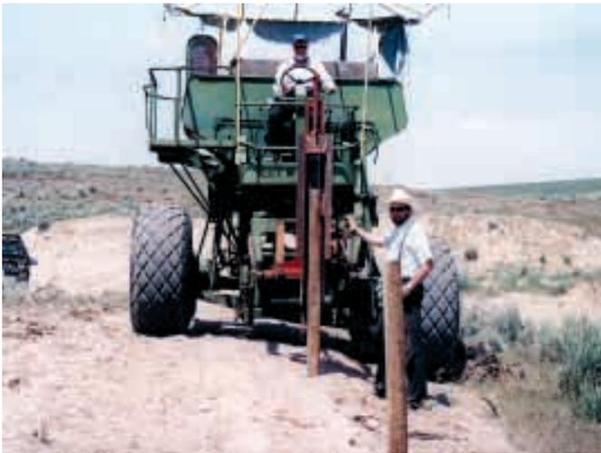
Post driver mounts in place of header. Hydraulics originally used for the reel lift raise and lower driver head, while the header cylinder raises the driver itself for transport.
