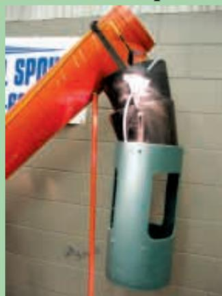
"Never spill" spout attaches to auger instead of grain bin and has a loud alarm that signals when bin is full.
