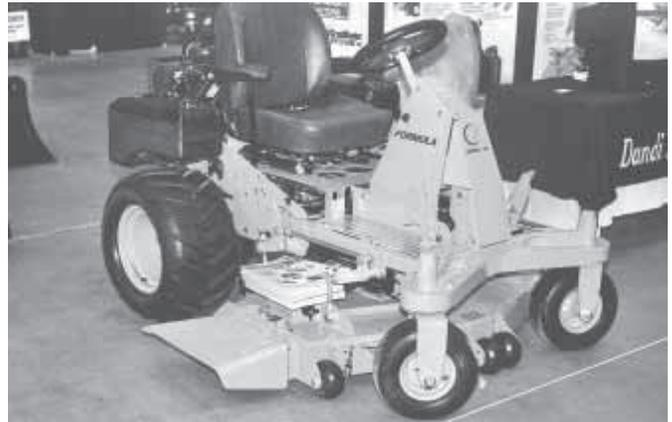
Two steerable caster wheels on front are linked to hydraulic motors on back. As wheels are cranked in either direction, power is adjusted to make a smooth turn. Front wheels have enough traction to handle hills.
