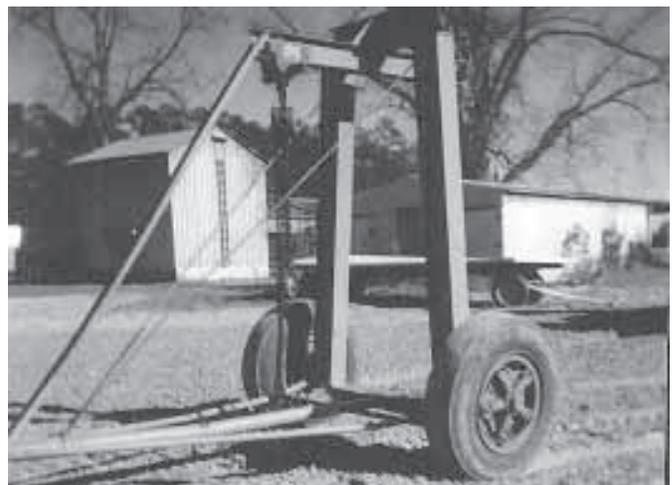
Frame and wheels are from a large truck's front end. Van Arnette added 8-in. I-beams from a scrap yard, and a 2 1/2-ton hoist and chain.
