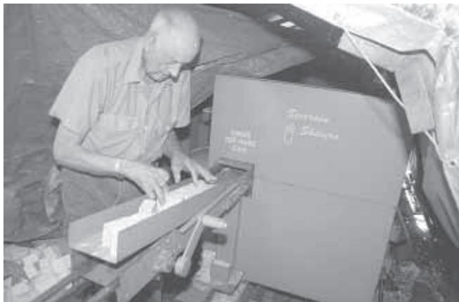
Harvey Severson feeds blocks of wood into the Severson Shaver, which turns a tray of wood into a big pile of wood curls in seconds.
