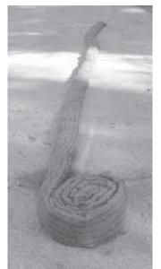
Absorbent "filtration pillow" is designed to intercept surface runoff of liquid manure and remove the nitrogen, before it gets into the environment.
