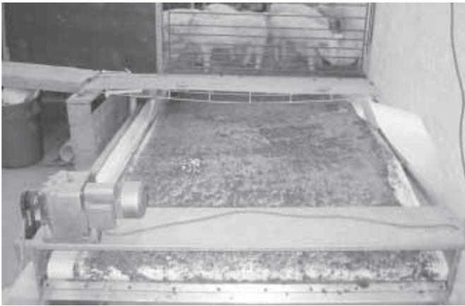
Conveyor belt runs length of barn beneath slatted portion of pens, moving manure out of barn. Belt is tilted at a 4 degree angle, so urine runs into channel along lower side.
