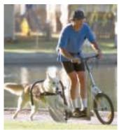
Adult-sized scooter has curved rear outrigger made from bicycle tubing, to which dog can be hamessed. A second or third outrigger can be added.
